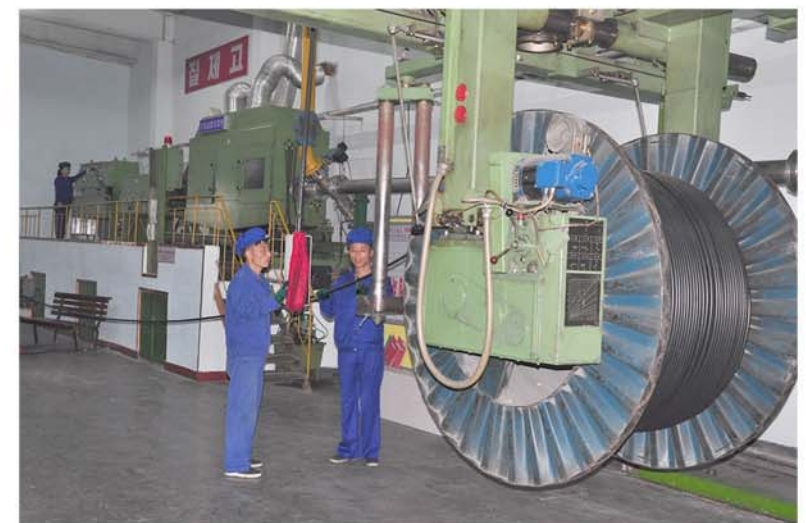
The production process of cross-linked polyethylene insulated power cable.
