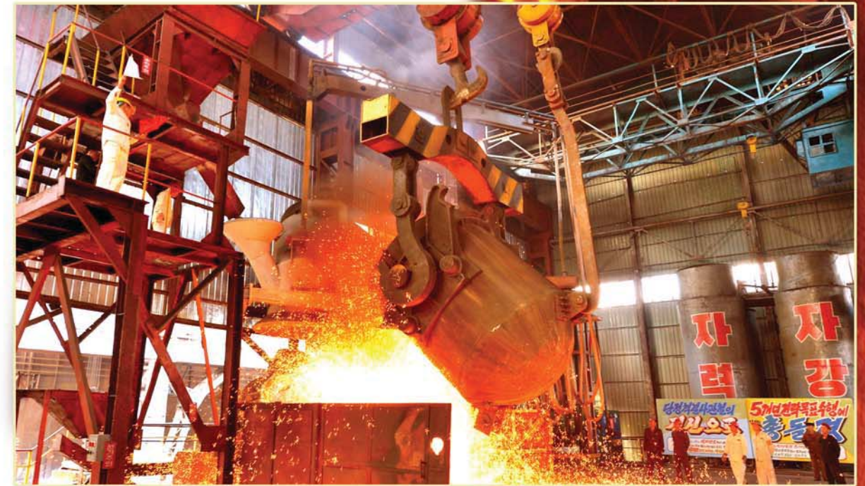
The oxygen-blown converter helps increase steel production.
