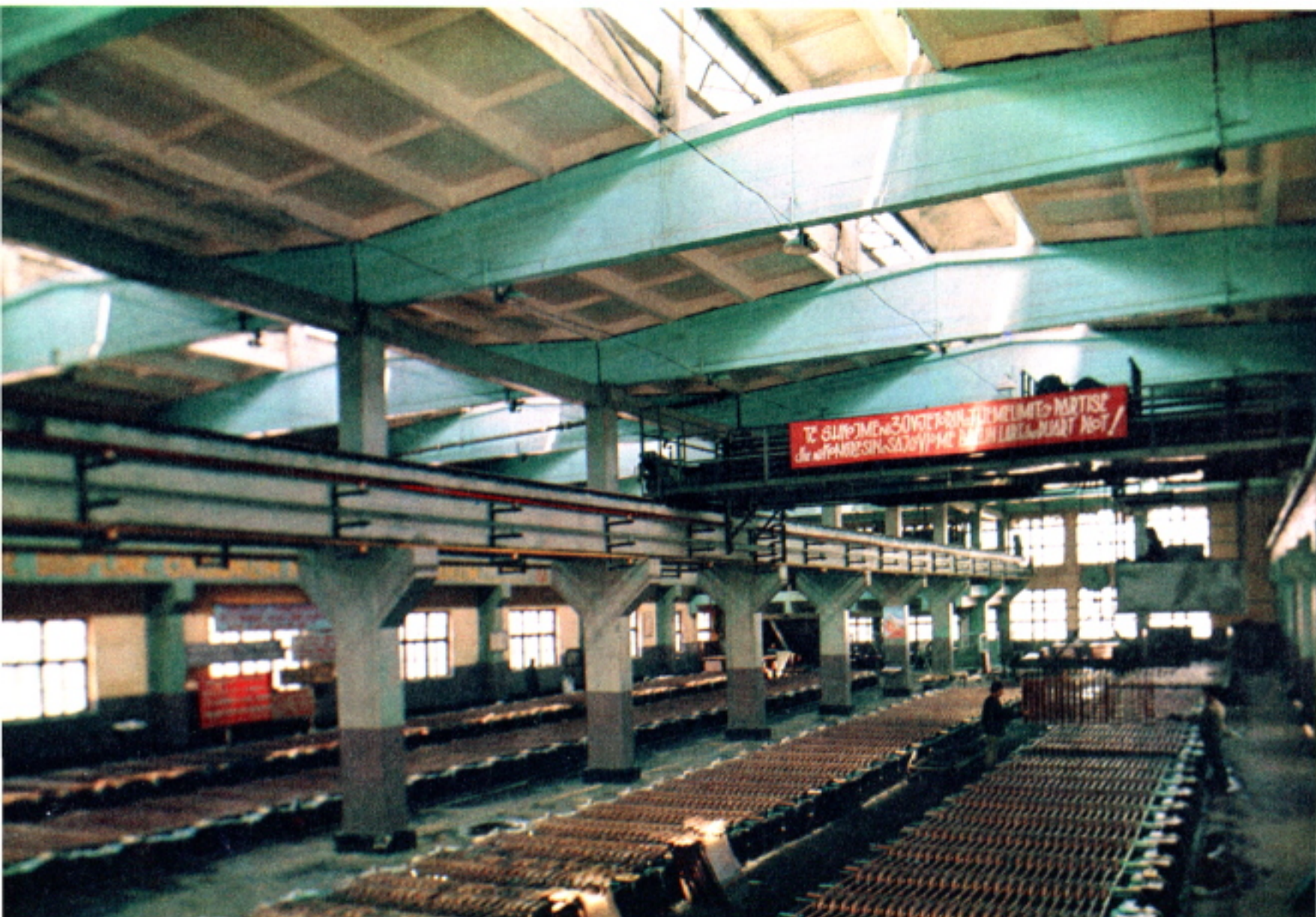
The electrolysis department in the Copper Refining and Processing Plant of Rubik.
