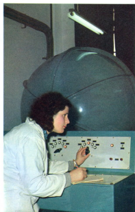
—The laboratory girl Suzanna Tigani operating the apparatus for measuring the light flux of lamps.
